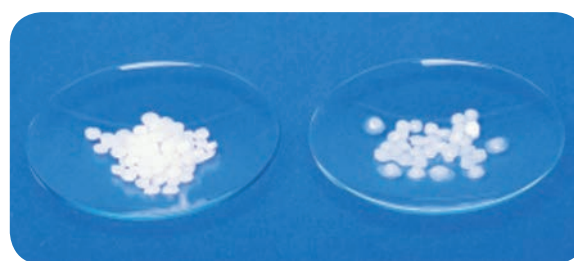
Figure 9.11 Deliquescence in Sodium hydroxide
